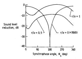
Fig. 7 Sound level reduction: x/a = 0,  $\theta = 0$ , and  $\Omega = 0.14$ .
