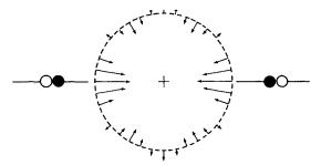
Fig. 8 Normalized radial intensity at the shell wall: x/a = 0,  $\phi_s = 0$  deg, and  $\Omega = 0.2$ .
