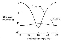
Fig. 11 Line power reduction at the shell wall: x/a = 0.
