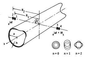
Fig. 1 Geometry, coordinate system, and model shapes.
