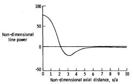
Fig. 10 Nondimensional line power flow at the shell wall:  $\phi_s = 0$  deg and  $\Omega = 0.2$ .
