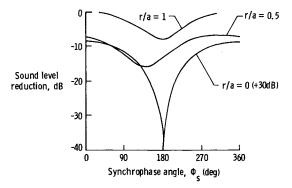
Fig. 6 Sound level reduction: x/a = 10,  $\theta = 0$ , and  $\Omega = 0.2$ .
