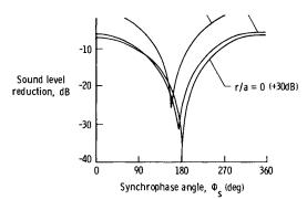
Fig. 5 Sound level reduction: x/a = 0,  $\theta = 0$ , and  $\Omega = 0.2$ .
