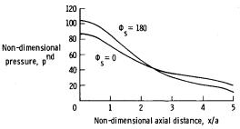
Fig. 2 Axial external pressure distribution: r/a = 1,  $\theta = 0$ , and  $\Omega = 0.2$ .
