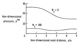
Fig. 3 Axial internal pressure distribution: r/a = 1,  $\theta = 0$ , and  $\Omega = 0.2$ .
