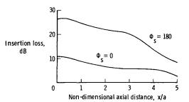
Fig. 4 Axial shell insertion loss:  $\theta = 0$  and  $\Omega = 0.2$ .
